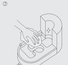
Clean the base with a soft cloth or the included cleaning brush to remove excess of mineral deposits. Make sure all parts are dry before reassembling your humidifier.
