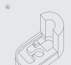
Remove the mist nozzle, mist tube, hot/cold mist mixer, noise silencer and float.
