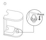
Place the water filter back into the tank. Make sure the water filter clicks in place.
