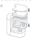
Put the water tank back in place and close the top cover.
