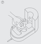
Clean the base with a soft cloth or the included cleaning brush to remove excess of mineral deposits. Make sure all parts are dry before reassembling your humidifier.
