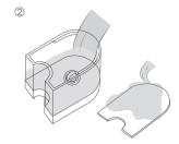
Detach the cover and water tank from the humidifier and clean thoroughly.
