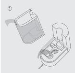
Drain any remaining water from the tank and the base.
